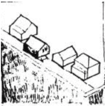
Too close to roadway
